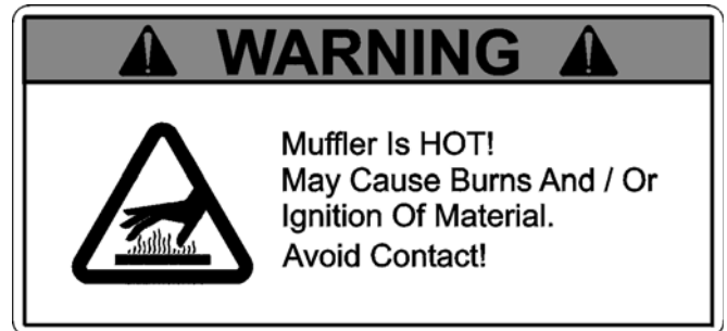
MUFFLER HOT, Front Side of Muffler Brace Right Side Top of Fan Shield P/N 169065 (Quantity (2))
