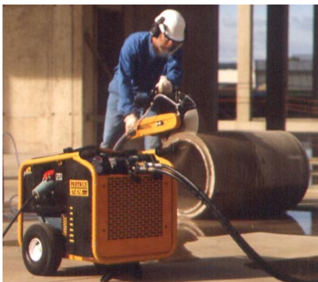
The HE 40/HP 40 are air-cooled and independent of water.
