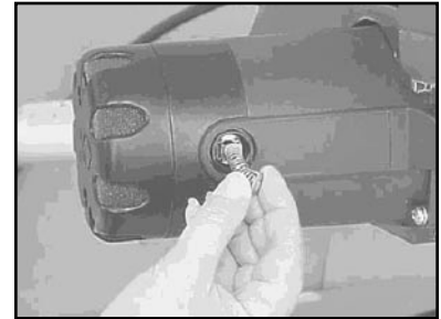
(C) Align and install the new Motor Brush
