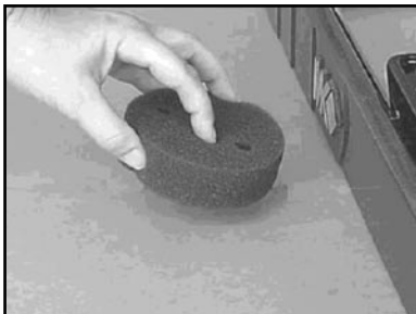
(D) Clean up Filter by tapping it on a hard surface or use compressed air.
