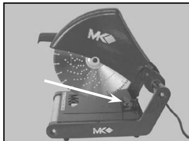
Position Back Stop in Backward Location and tighten both the knob and wing nut
