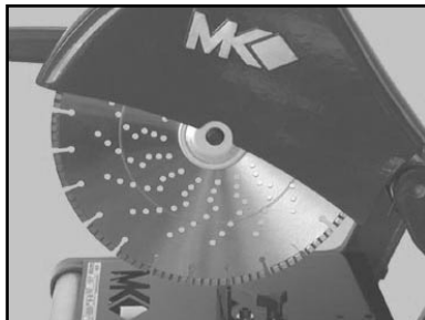
(D) Install the Diamond Blade onto Blade Shaft. Ensure that it is seated properly on the Flange.
