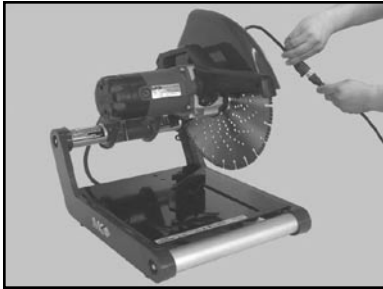
(A) Unplug the PX-3 from its Power Source
