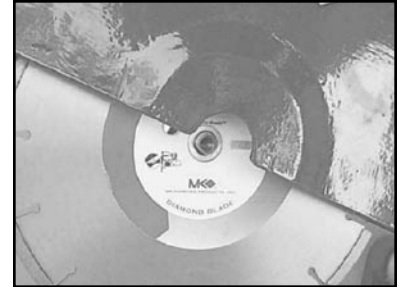
(C) Install and seat Blade –verify rotation.
