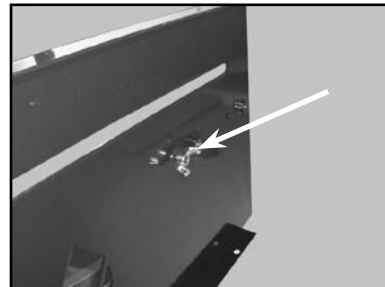
Loose wingnut located underneath the table
