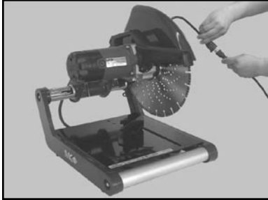
(A) Unplug the PX-3 from Power Source
