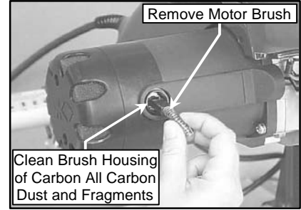
(C) Remove Motor Brush and Clean Brush Housing
