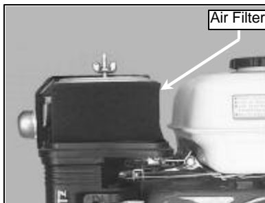
(E) Clean engine Air Filter (See Engine Air Filter Inspection Cleaning and Replacement)
