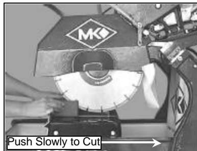
(H) Slowly push piece toward the blade – continue until the cut is complete
