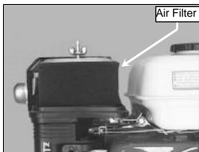
(A) Replace engine Air Filter (See Engine Air Filter Inspection Cleaning and Replacement)
