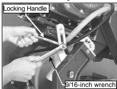
(A) Remove Cutting Head Locking Handle from shipping location discard the Shipping Nut
