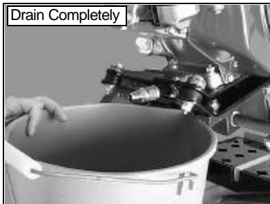
(C) Drain Oil (conform to Federal, State and Local laws for disposal)
