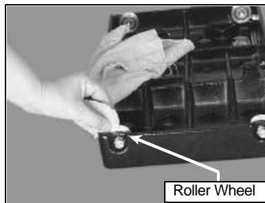
(H) Clean Movable Cutting Table Roller Wheels
