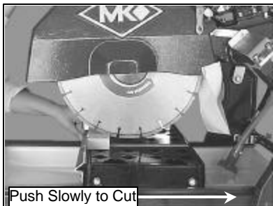
(F) Cut the Dressing Stick 7 or 8 times to dress the Blade
