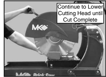
(J) Continue lowering the Cutting Head until the cut is complete raise the cutting head when the cut is complete
