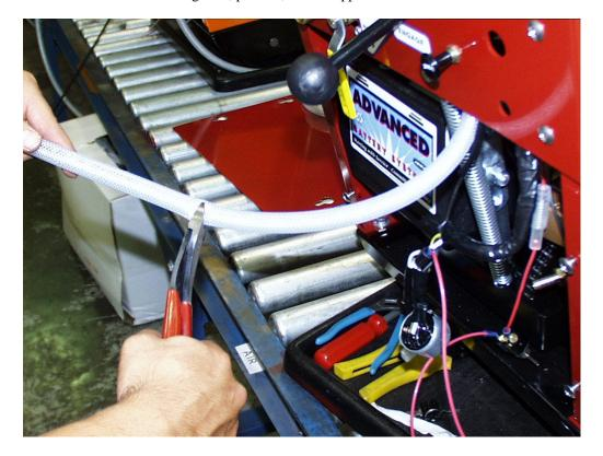
7. Attach loose part of hose to outlet fitting of water pump and install pump. Attach ground wire when installing pump to mounting screw.
