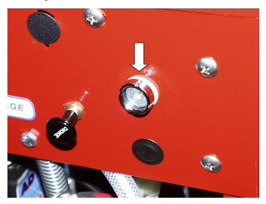
4. Pull ignition switch out and separate white wires
