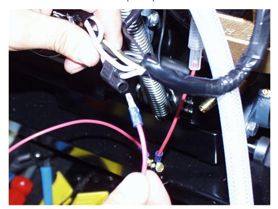
10. Re-install ignition switch, and install water pump switch. Water pump will be shipped in the off position which is to point down when installed.
