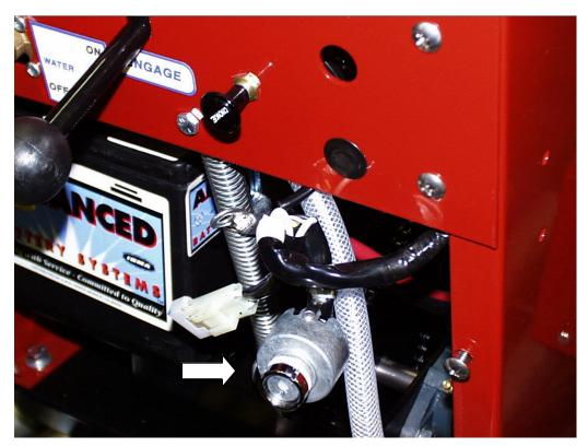
5. Connect bullet clamp-on receptacle to white wire
