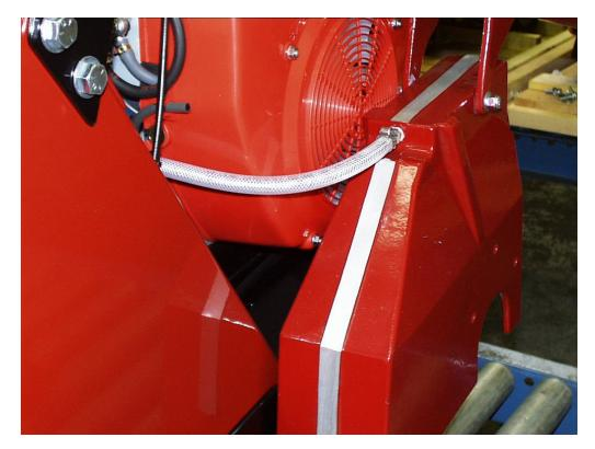
12. Secure loose wires away from drive chain and re-install rear panel.
