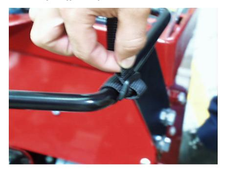
3. Insert strap into upper slot of plastic slide as shown.
