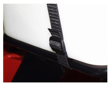
5. Install water tank and buckle strap. Adjust by pulling slack after buckling. When removing water tank it is necessary to give buckle slack and re-adjust when buckling
