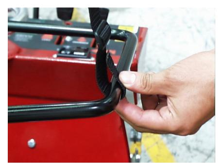
2. Insert strap into lower slot of plastic slide as shown.
