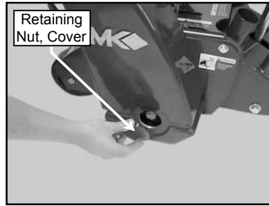
(H) Install the Shaft, Retaining Nut Cover onto the Belt Guard
