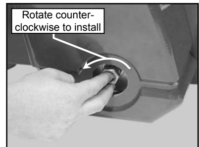
(C) Install the Shaft, Inner Retaining Nut
