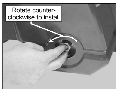
(M) Install the Shaft, Outer Retaining Nut
