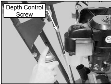
(J) Lubricate Clean the Depth Control Screw
