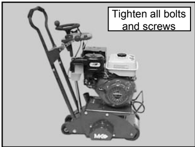
(A) Verify the tightness of all bolts and screws found on the SG-2
