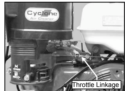
(F) Clean engine throttle linkage with a dry cloth
