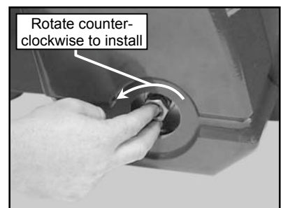
(F) Install the Shaft, Outer Retaining Nut
