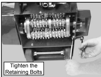
(J) Tighten the Shaft Guard Cover Retaining Bolts using 9/16 wrenches and/or sockets
