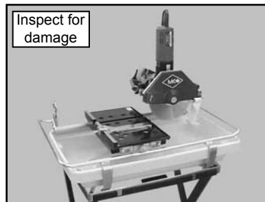
(E) Inspect the MK-770 for damage – ensure the cord is free of cracks or cuts
