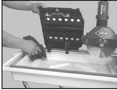
(J) Clean the Adjustable Cutting Guide, Guide Bar
