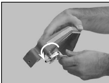
(I) Remove the Blade Guard Intake Fitting
