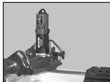
(K) Tighten the Blade Guard, Retaining Knob
