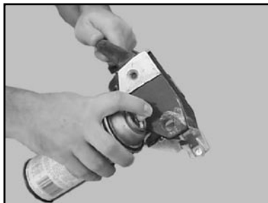
(J) Lubricate the Cutting Head Pivot Holes
