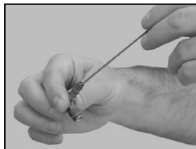
(J) Clean the Blade Guard Intake Fitting
