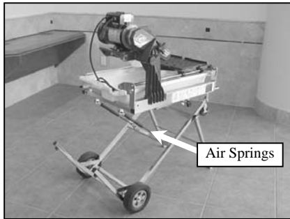
(M) Air Springs are fully extended and saw is in Horizontal position
