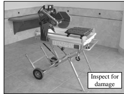
(E) Inspect the MK-101 for damage – ensure the cord is free of cracks or cuts
