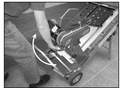
(L) Pull from the Cutting Head Handle until Air Springs are fully extended
