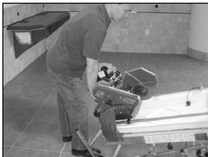
(D) Push down on Cutting Head until Air Springs are fully compressed
