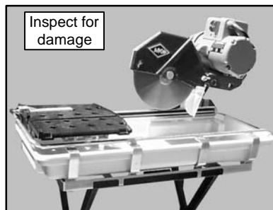
(E) Inspect the MK-101 for damage – ensure the cord is free of cracks or cuts
