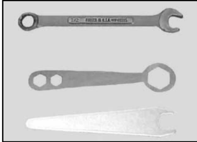
1/2-inch Wrench or MK Triple Hole Box Wrench and MK Open End Wrench
