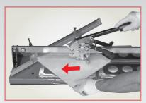
CUTTING: Score the cutting wheel once on ceramic tile, by means of sliding arm.
