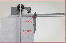
$90^{\circ}$  ADJUSTMENT: Adjust the ruler to  $0^{\circ}$  position by means of turning around its axis and fix it. Adjust the dimension you want to cut by means of the sliding angle on the ruler and read the dimension from the bottom scala.
