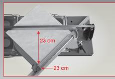
$45^{\circ}$  ADJUSTMENT: Adjust the ruler to  $45^{\circ}$  position by means of turning around its axis and fix it. Adjust the dimension you want to cut by means of the sliding angle on the ruler and read the dimension from the upper scala.
