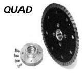
As an option the Plus comes drilled in a special version called Quad Drive. This permits mounting on angle grinders when you would like to cut "flush". The Quad adapter eliminates the need for the lock nut which would normally prevent you from flat cutting operations. Great for tight spots.
